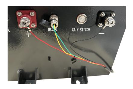
Battery Side: Red: + Main Positive Plug into RS485
